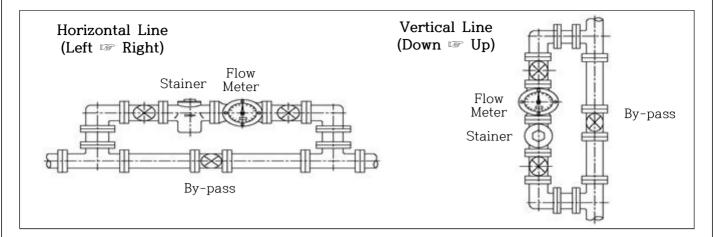
Flow altering device such as elbows, valves and reducers can affect accuracy.
